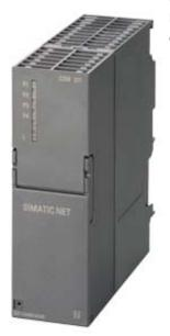
Compact Switch Module CSM 377 Connection SIMATIC S7-300 and up to 3 further nodes to Industrial Ethernet with 10/100 Mbit/s unmanaged switch, 4 RJ45 ports, External 24 V DC power supply LED diagnostics, S7-300 module, incl. electron. Equipment Manual on CD-ROM
