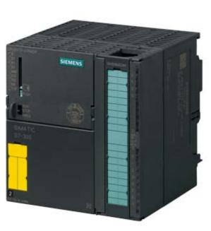
SIMATIC S7-300, CPU 317TF-3 PN/DP, Central processing unit for PLC, Technology and safety tasks, 1.5 MB work memory, 1st interface MPI/DP 12 Mbit/s, 2nd interface DP (drive), 3rd interface Ethernet PROFINET with 2-port switch, Integr. I/O for technology, Front connector (1x 40-pole) and Micro Memory Card min. 8 MB required
