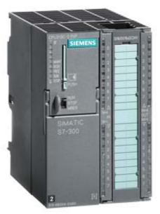
SIMATIC S7-300, CPU 313C-2 PTP Compact CPU with MPI, 16 DI/16 DO, 3 high-speed counters (30 kHz), integrated interface RS485, Integr. power supply 24 V DC, work memory 128 KB, Front connector (1x 40-pole) and Micro Memory Card required
