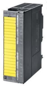
SIPLUS S7-300 SM336 F 6AI 15 bit -25...+60 °C (70 °C with forced convection) With conformal coating Based on 6ES7336-4GE00-0AB0 . Fail-safe analog inputs For SIMATIC Safety, with HART support, up to Category 4 (EN 954-1) /SIL3 (IEC 61508)/ PLE (ISO 13849), 1x 20-pole
