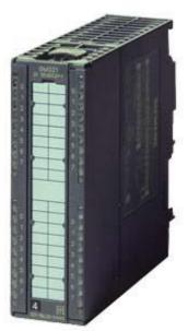
SIPLUS S7-300 SM 321-20-pole -25...+70°C with conformal coating Conformity with EN 50155 T1 Kat 1 Kl A/B based on 6ES7321-7BH01-0AB0. Digital "input Isolated ""16 DI; 24 V DC," "1x 20-pole,"" process interrupt," diagnostics, suitable for isochronous mode operation
