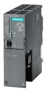
SIPLUS S7-300 CPU 317F-2PN/DP -25...+60°C with conformal coating based on 6ES7317-2FK14-0AB0 . Central processing unit with 1.5 MB work memory, 1st interface MPI/DP 12Mbit/ s, 2nd interface Ethernet PROFINET, with 2-port switch, Micro Memory Card required
