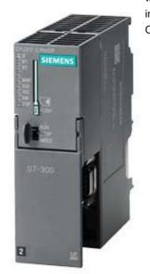
SIPLUS S7-300 CPU 317-2PN/DP -25...+70°C with conformal coating based on 6ES7317-2Ek14-0AB0 . Central processing unit with 1 MB work memory, 1st interface MPI/DP 12Mbit/ s, 2nd interface Ethernet PROFINET, with 2-port switch, Micro Memory Card required
