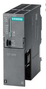
SIPLUS S7-300 CPU315-2PN/DP -25 ... +70°C with conformal coating based on 6ES7315-2EH14-0AB0 . CENTRAL PROCESSING UNIT WITH 384 KBYTE WORKING MEMORY, 1. INTERFACE MPI/DP 12MBIT/S, 2. INTERFACE ETHERNET PROFINET, WITH 2 PORT SWITCH, MICRO MEMORY CARD NECESSARY
