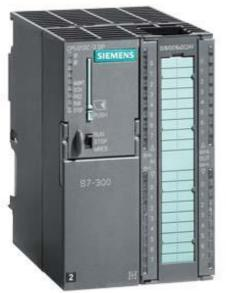
SIPLUS S7-300 CPU CPU 313C-2DP with conformal coating according to EN 50155 T1 Cat 1 Cl A/ B based on 6ES7313-6CG04-0AB0 . Compact CPU with MPI, 16 DI/16 DO, 3 high-speed counters (30 kHz), integrated DP interface, Integr. power supply 24 V DC, work memory 128 KB, Front connector (1x 40-pole) and Micro Memory Card required
