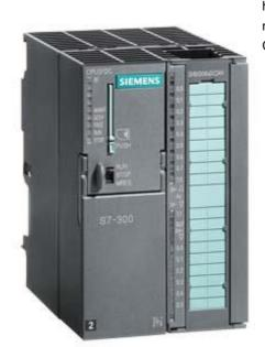
SIPLUS S7-300 CPU 312C for medial exposure -25...+70°C based on 6ES7312-5BF04-0AB0 . Compact CPU with MPI, 10 DI/6 DQ, 2 high-speed counters (10 kHz) Integr. power supply 24 V DC, work memory 64 KB, Front connector (1x 40-pole) and Micro Memory Card required
