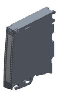
SIMATIC S7-1500 Analog output module AQ 2x U/I ST, 16 bit resolution, accuracy 0.3%. 2 channels in groups of 2; Diagnostics; Substitute value; Delivery including push-in front connector, infeed element, shield bracket and shield terminal
