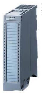
SIMATIC S7-1500 analog input module AI 8xU/I HS, 16 bit resolution, accuracy 0.3% 8 channels in groups of 8; common mode voltage 10 V; Diagnostics; Hardware interrupts 8 channels in 0.0625 ms Oversampling; Delivery including infeed element, shield bracket and shield terminal: Front connector (screw terminals or push-in) to be ordered separately
