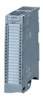
SIMATIC S7-1500 analog input module AI 8xU/I HF, up to 24 bit resolution, accuracy 0.1%, 8 channels in groups of 1; common mode voltage: 30 V AC/60 V DC, Diagnostics; Hardware interrupts Measured values scalable, measuring range adjustment, Calibrate in RUN; Delivery including infeed element, shield bracket and shield terminal: Front connector (screw terminals or push-in) to be ordered separately
