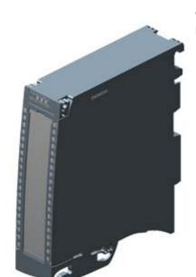
SIMATIC S7-1500, digital output module DQ 32x24 V DC/0.5 A HF; 32 channels in groups of 8; 4 A per group; Single-channel diagnostics; Substitute value: Front connector (screw terminals or push-in) to be ordered separately
