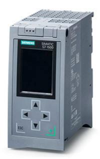
SIMATIC S7-1500F, CPU 1516F-3 PN/DP, Central processing unit with work memory 1.5 MB for program and 5 MB for data, 1st interface: PROFINET IRT with 2-port switch, 2nd interface: PROFINET RT, 3rd interface: PROFIBUS, 10 ns bit performance, SIMATIC Memory Card required
