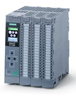
\*\*\* Spare part \*\*\* SIMATIC S7-1500 compact CPU CPU 1512C-1 PN, Central processing unit with work memory 250 KB for program and 1 MB for data, 32 digital inputs, 32 digital outputs, 5 analog inputs, 2 analog outputs, 6 high-speed counters, 4 high-speed counters for PTO/PWM/frequency output 1st interface: PROFINET IRT with 2-port switch, 48 ns bit performance, incl. push-in front connector, SIMATIC Memory Card required
