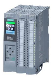
SIMATIC S7-1500 Compact CPU CPU 1511C-1PN, central processing unit with working memory 175 KB for program and 1 MB for data, 16 digital inputs, 16 digital outputs, 5 analog inputs, 2 analog outputs, 6 high speed counters, 4 high speed outputs for PTO/PWM/frequency output 1. interface: PROFINET IRT with 2 port switch, 60 NS bit-performance, incl. front connector push-in, SIMATIC memory card necessary
