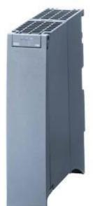
SIPLUS S7-1500CM PtP RS422/485 -40...+70°C start up -25°C with conformal coating based on 6ES7541-1AB00-0AB0 . Communication module for Serial connection RS422 and RS485, Freeport, 3964 (R), USS, MODBUS RTU Master, Slave, 115200 Kbit/s, 15-Pin D-sub socket
