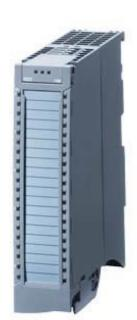
SIPLUS S7-1500 AO 4xU/I ST -40 °C ... +70°C with conformal coating based on 6ES7532-5HD00-0AB0 . Analog output module 16 bit resolution, Accuracy 0.3%. 4 channels in groups of 4, "diagnostics; substitute value" incl. infeed element, shield bracket and shield terminal
