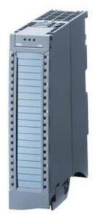
SIPLUS S7-1500 AI 8xU/I HS -40 °C ... +70°C with conformal coating based on 6ES7531-7NF10-0AB0 . Analog input module AI 8xU/I HS, 16 bit resolution, Accuracy 0.4% 8 channels in groups of 8, "Common mode voltage 10 V;" "diagnostics; hardware" "interrupts"" 8 channels in 0.125" ms incl. infeed element, Shield bracket and shield terminal
