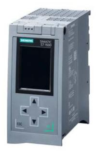
SIPLUS S7-1500 CPU-1516F-3 PN/DP -25...+60°C start up -20 °C with conformal coating based on 6ES7516-3FN01-0AB0. Central processing unit with RAM 1.5 MB for program and 5 MB for data, 1st interface: PROFINET IRT with 2-port switch, 2nd interface: Ethernet, 3rd interface: PROFIBUS, 10 ns bit performance, SIMATIC Memory Card required
