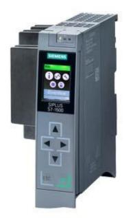
SIPLUS S7-1500 CPU 1513-1 PN -40...+70°C start up -20°C with conformal coating based on 6ES7513-1AL01-0AB0 . Central processing unit with Work memory 300 KB for program and 1.5 MB for data, 1st interface: PROFINET IRT with 2-port switch, 40 ns bit performance, SIMATIC Memory Card required
