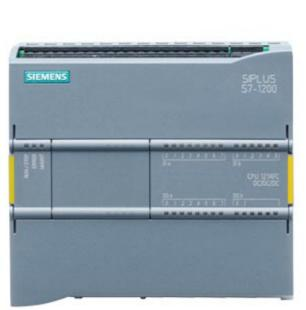
SIPLUS S7-1200 CPU 1214FC DC/DC/relay -25...+55°C with conformal coating based on 6ES7214-1HF40-0XB0 . compact "CPU, DC/DC/relay, ""onboard I/O:" "14 DI 24 V DC;"" ""10 DO relay 2" "A;"" 2 AI 0-10 V DC, Power" supply: DC 20.4-28.8 V DC Program/data memory 125 KB
