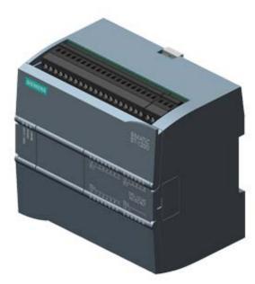
SIPLUS S7-1200 CPU 1214C AC/DC/relay -40...+60°C with conformal coating Signal board usable based on 6ES7214-1BG40-0XB0 . compact CPU, AC/DC/relay, onboard I/O: "14 DI 24 V DC; 10 DO relay 2 A;" 2 AI 0-10 V DC, Power supply: AC 85-264 V AC @ 47-63 Hz, Program/data memory 100 KB
