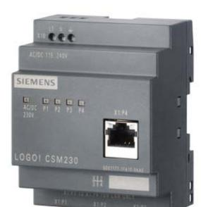
LOGO! CSM 230 Compact Switch Module of connection of a LOGO! (... 0BA7) and up to 3 further nodes to Industrial Ethernet with 10/100 Mbit/s; unmanaged switch, 4 RJ45 ports, 1x front port for diagnostics AC/DC 115 ... 240 V
